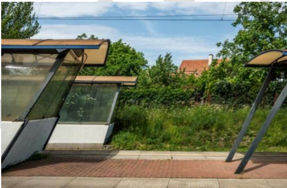
Figure 4. Image skew caused by a sensor with a rolling shutter. [12]
