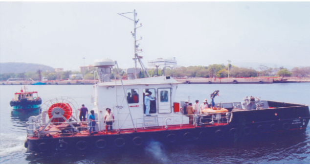
M.V.JALSUDHAK, (Oil Recovery-cum-Pollution Control Vessel) Visakhapatnam Port Trust
