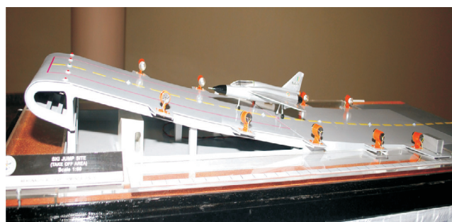
Shore Based Test Facility (SBTF)
